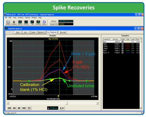
**Figure 1.** Spectral data shows equal response for a Mg spike in a 1% HCl standard and 30% brine.
