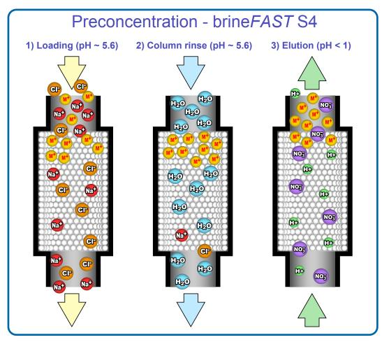
**Figure 4.** At a pH  $\sim$  5.6, many metals are chelated on the preconcentration column, while matrix elements are flushed from the column. Metals are eluted directly to the ICP with nitric acid.
