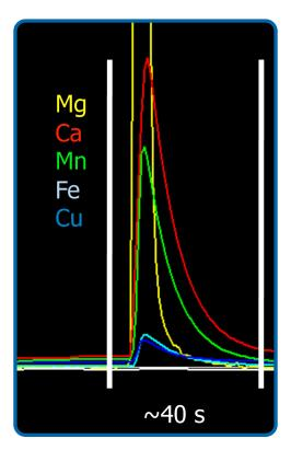
**Figure 5.** Simultaneous elution profiles for preconcentration elements allows simple quantification after matrix removal
