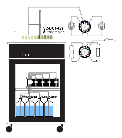
Figure 2. brine FAST S4 system schematic
