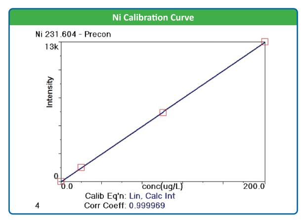
**Figure 9.** Typical calibration curve for 50% Caustic Soda (10x diluted) demonstrating linearity at higher concentrations. If needed, higher level calibrations at the ppm level are also linear.
