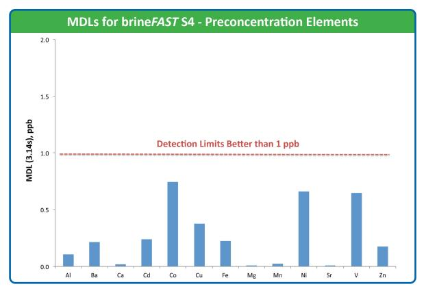
**Figure 10.** MDLs better than 1 ppb were achieved for preconcentration mode elements (0.5 ppb, n=7, 3.14 $\sigma$ )
